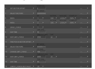
In the WebMotion® menu "program" the different force functions of I\_FORCE CALIBRATION, I\_FORCE LIMITATION and I\_FORCE MONITORING can be combined and defined with the use of the according commands.
