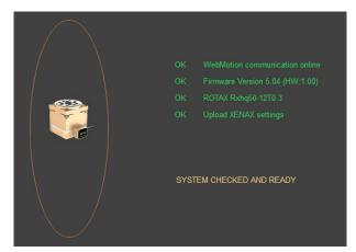
If the XENAX® servo controller does not recognize a LINAX® or ELAX® linear motor axis or a ROTAX® rotary axis, XENAX® assumes a connection with third party motor. Instead of "Go Pos 0" WebMotion® offers Jog + und Jog – functions.
