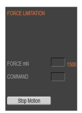
Motion with limited force to an object or end position if no objects are present (e.g. insert parts). Or move with very little force to detect the "object touching position".
